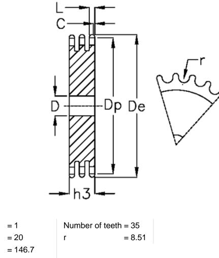
C = 1 D = 20 De = 146.7 Dp = 141.68 For chain size =  $1/2 \times 5/16$ For chain type = 08 B-3 h3 = 34.9 L = 7
